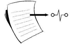
The selected output is turned on, turned off, or turned on for a selected amount of time. The function is now completed and the next line of the page is executed. Note: The page will begin the next line even if the output is timed on.
